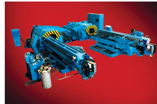
Centrifugal casting machine (Courtesy Gibson Centritech Ltd.)
