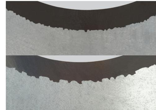
Comparison micrograph of interface rough vs. textured liner
